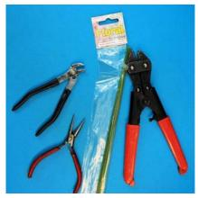
The tools in the photo are a needle-nose pliers, a heavy-duty wire cutter and an ignition pliers (found in the auto dept of Sears or any auto store). They will bend a wire completely closed. They are very useful for many doll related chores.
